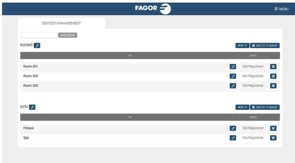
Once the devices have been created in Ikusi Flow, TV screens will show the registration menu. Use the TV (or FLOW STB) remote control to associate an existing device to one of the devices created in Ikusi Flow, following these steps in the TV screens:
