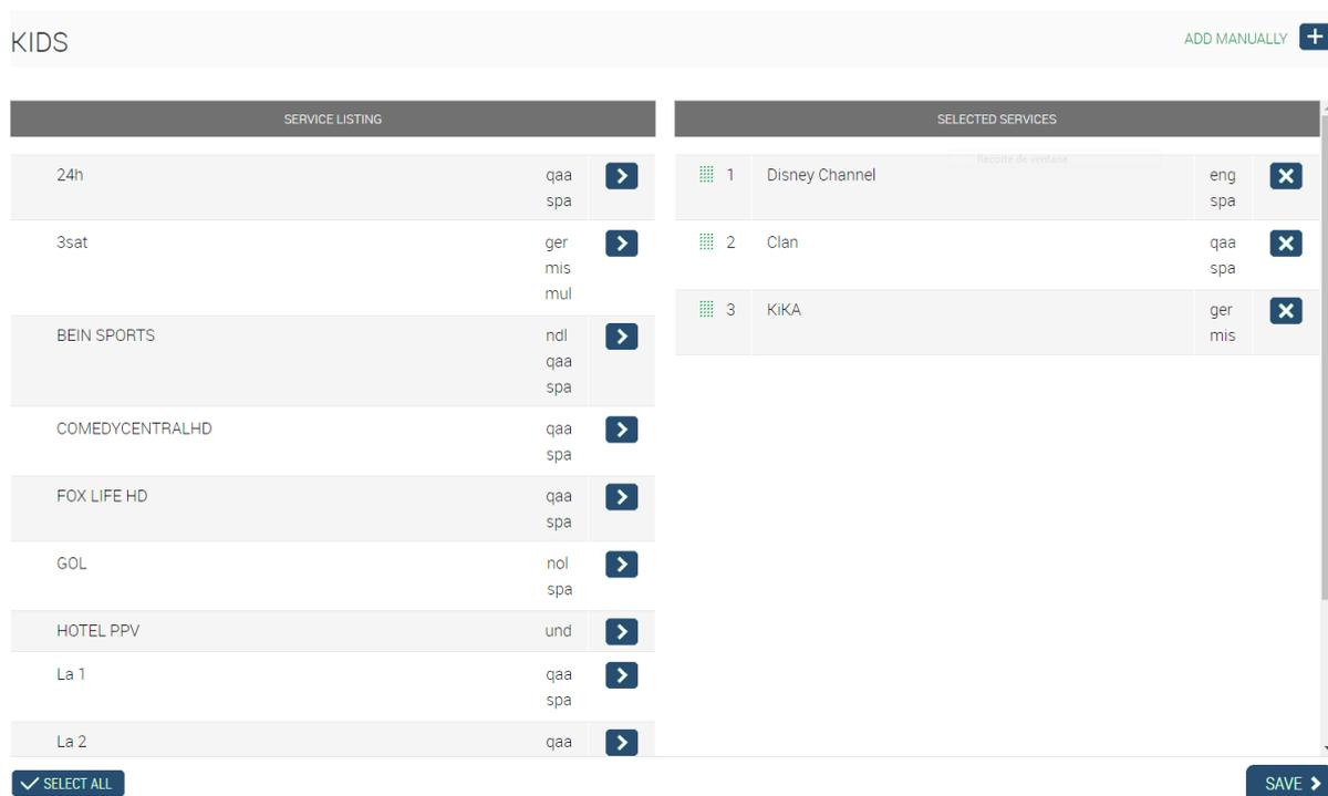
Finally, Device Manager allows the integration of external IP services (coming from 3rd party systems) for management in the same network. To add the information of external IP services, select ADD MANUALLY to open the fields to fill and set Service Name, IP address and Port. Once done, push SAVE AND ADD button.
